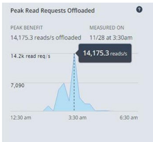
At peak times, over 14,000 IOPS from the VDI environment are being offloaded from Bartlett’s EqualLogic arrays.
